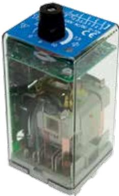
Plug-in electronic railway timer relay with 4 change-over contacts. When the relay is not energized anymore, there is a delay on drop-out, without any auxiliary power supply.
