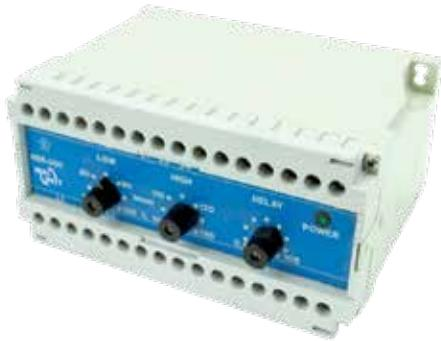
Over- and undervoltage monitoring railway relay with two change-over contacts. Suitable for 3-phase 400 VAC 50 Hz. When the relay is activated, there is a delay on pull-in.
