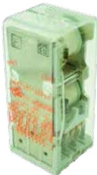
Latching, safety-critical railway relay with 2 stable magnetic latched states. When 1 coil is energized, the relay actuates from magnetically latched position 1 to 2. When the other coil is energized, the relay actuates back to position 1.
