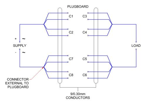
POLARITIES SHOWN  $\underline{\text{MUST}}$  BE OBSERVED WHEN USING A DC SUPPLY
