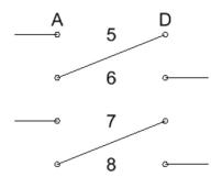
THIS ARRANGEMENT <u>MUST</u> BE USED TO GIVE DETECTION OF A WELDED HEAVY DUTY FRONT CONTACT
