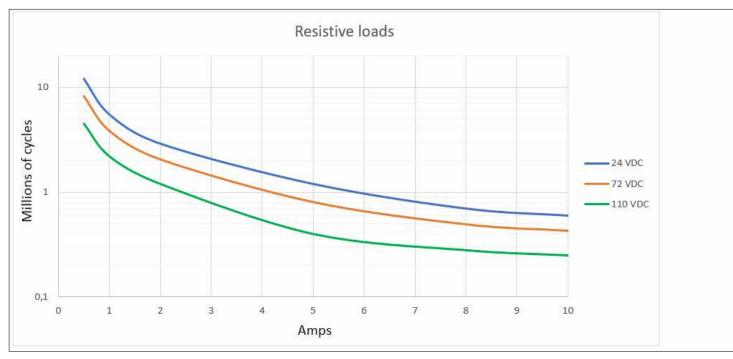
By connecting 2 contacts in series the DC current breaking capacity is increased by 50 %. Electrical lifetime is tested under laboratory conditions with switching frequency 0.33 Hz.
