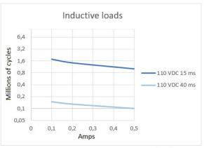
By connecting 2 contacts in series the DC current breaking capacity is increased by 50 %. Electrical lifetime is tested under laboratory conditions with switching frequency 0.33 Hz.
