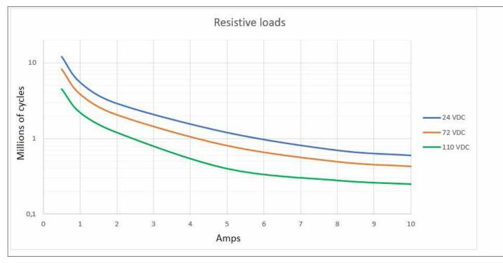
By connecting 2 contacts in series the DC current breaking capacity is increased by 50 %. Electrical lifetime is tested under laboratory conditions with switching frequency 0.33 Hz.
