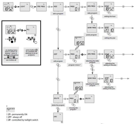
By shortly pressing @, you can toggle between the program number and the display of its settings. Use to toggle preset programs. By holding 👁 you can proceed with the required step - CHRNGE / DELETE. If you do not want to proceed, press 🌚 to go to the main settings without any change.
