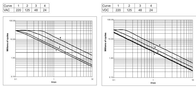
DC Current breaking capacity at L/R = 0
