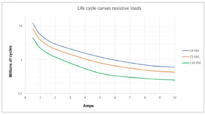
By connecting 2 contacts in series the DC current breaking capacity is increased by 50 %. Electrical lifetime is tested under laboratory conditions with switching frequency 0.33 Hz.
