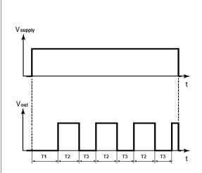
When supply voltage is applied, after period T1 the relay is activated for period T2.
