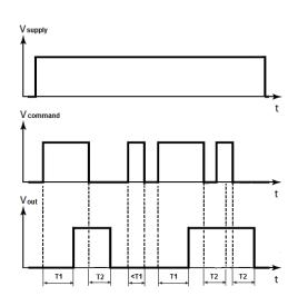
Supply voltage is applied to the relay. When command voltage is applied, after period T1 the relay is activated if the command voltage is supplied during T1.
