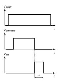
Supply voltage and command voltage is applied to the relay. The relay is activated for period T when command voltage is removed.
