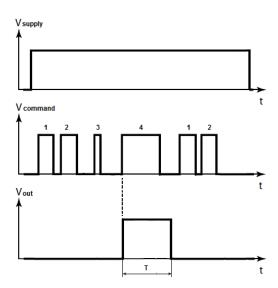
Supply voltage is applied to the relay. The  $4^{\text{th}}$  time a command voltage is applied regardless of the duration of the command voltage, the relay is activated for period T regardless the command voltage.
