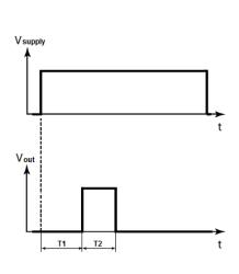
When supply voltage is applied, after period T1 the relay is activated once for period T2.
