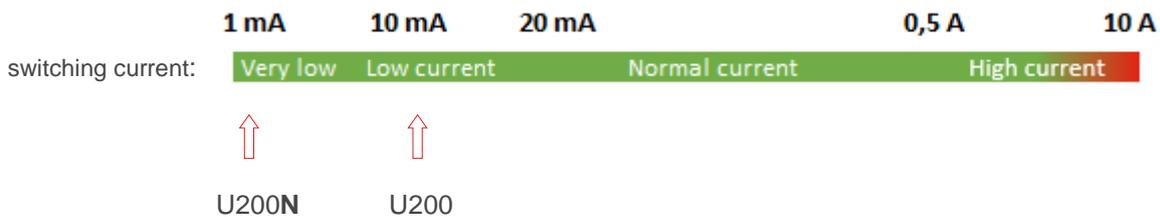
Advise to always use gold plated contacts when switching very low currents to prevent contact corrosion (option E).
