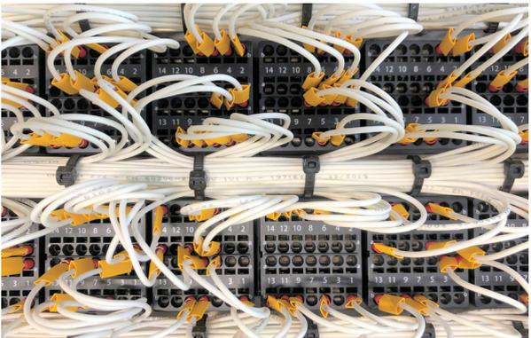
**Mechanical keying relay and socket (optional)**
