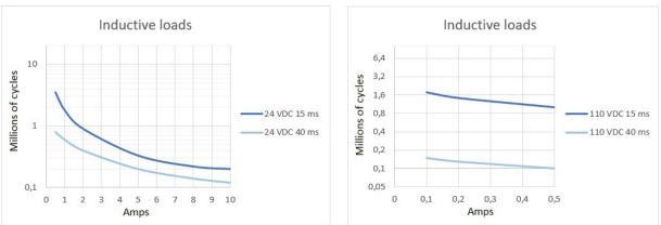
By connecting 2 contacts in series the DC current breaking capacity is increased by 50 %. Electrical lifetime is tested under laboratory conditions with switching frequency 0.33 Hz.
