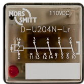
Red or green LED coil indicator
