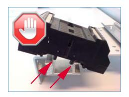
The new V23 & V29 sockets are equipped with 6 small pillars. The purpose of these pillars is to offer extra stability when the socket is wall mounted, but are unnecessary when the socket is mounted on a TH 35-15 rail.
