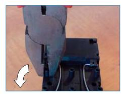
The pillars will have to be removed before the socket will fit on a TH 35-15 rail.
