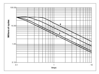
DC Current breaking capacity at L/R = 0
