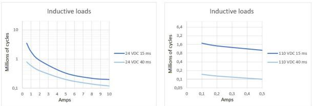
By connecting 2 contacts in series the DC current breaking capacity is increased by 50 %. Electrical lifetime is tested under laboratory conditions with switching frequency 0.33 Hz.
