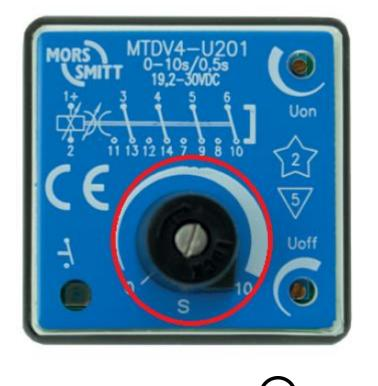
Turn knob fully counter clockwise <sup>4</sup> J until its stop.
