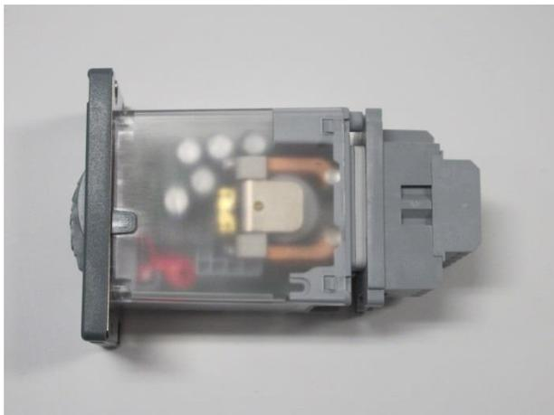
Relay plugged into a terminal block
