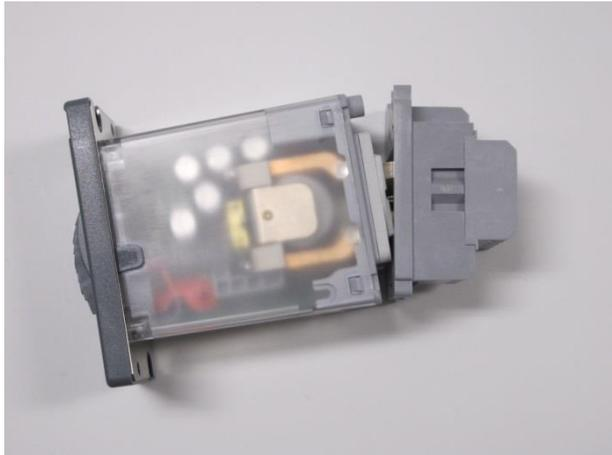
Relay partially removed from terminal block
